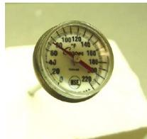
A thin stem thermometer with a range of 0°F - 220°F must be present to monitor temperatures.
